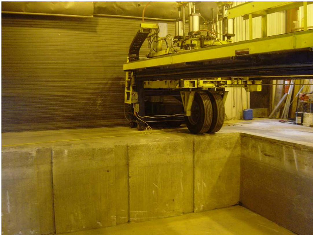
Figure 3.1.2: Picture of empty test pit and APT loading system.
